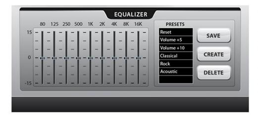
The EQ comes with 5 presets. You can add or delete or change presets as to meet your needs by using the corresponding buttons on the right hand side of this window.
